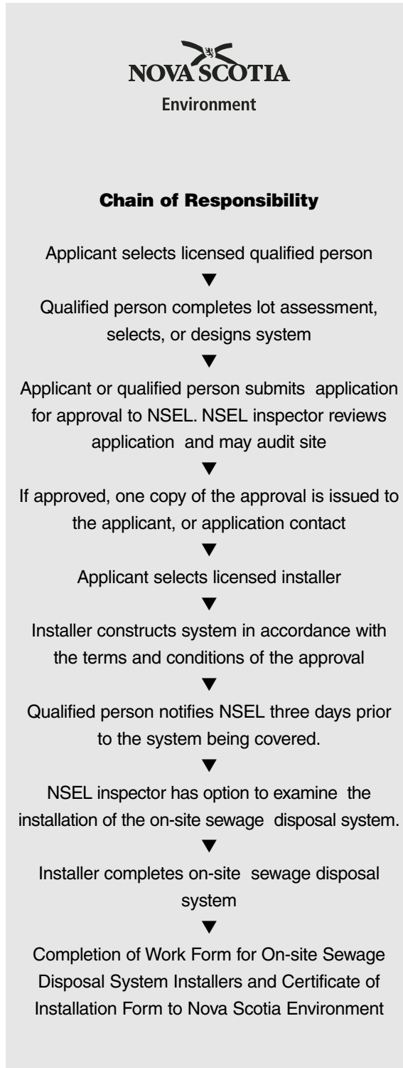
Figure 4 Approval Procedure Flowchart for an On-site System
