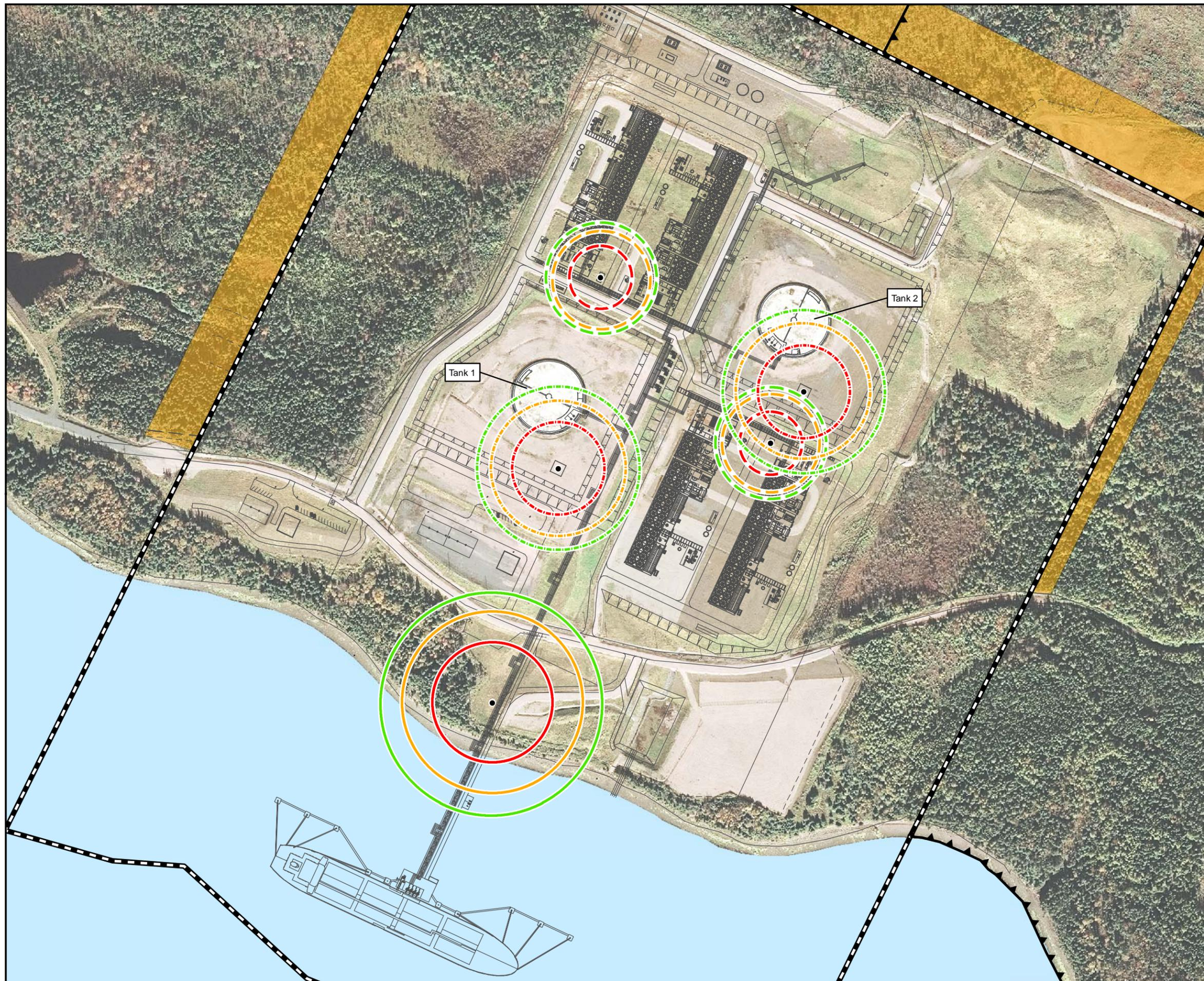
This design spill, which is defined in the next section, would flow into the basin localized within the bermed area of each tank. As shown on Map 2, the 5 kW/m<sup>2</sup> level doesn't go beyond the property limit, so this case is in compliance with the requirement of the CSA Z276 Standard.
