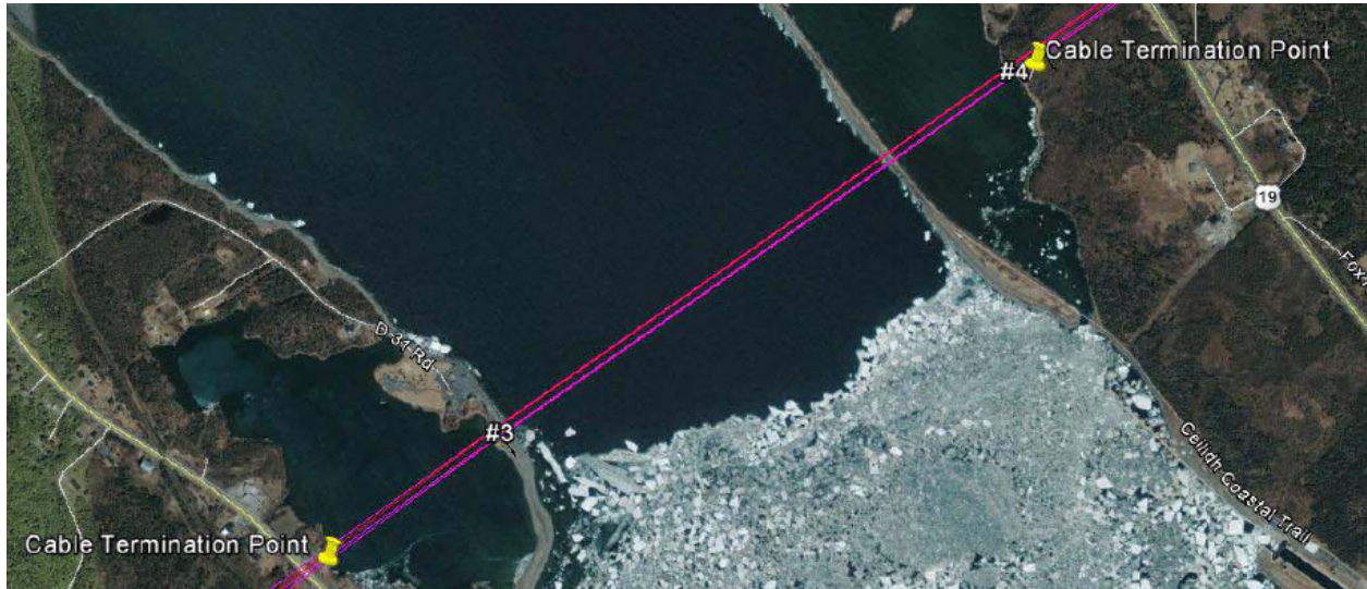
Figure 1 Submarine Cable Installation - Strait of Canso
