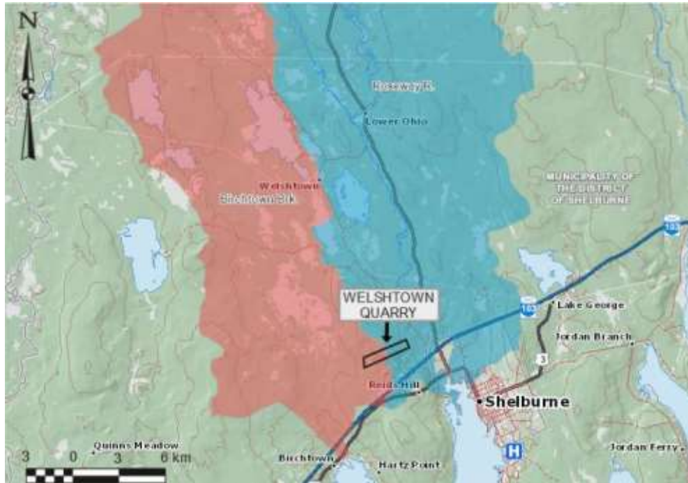
Figure 8. Welshtown Quarry property is divided by two sub-watersheds: Birchtown Brook and Roseway River.
