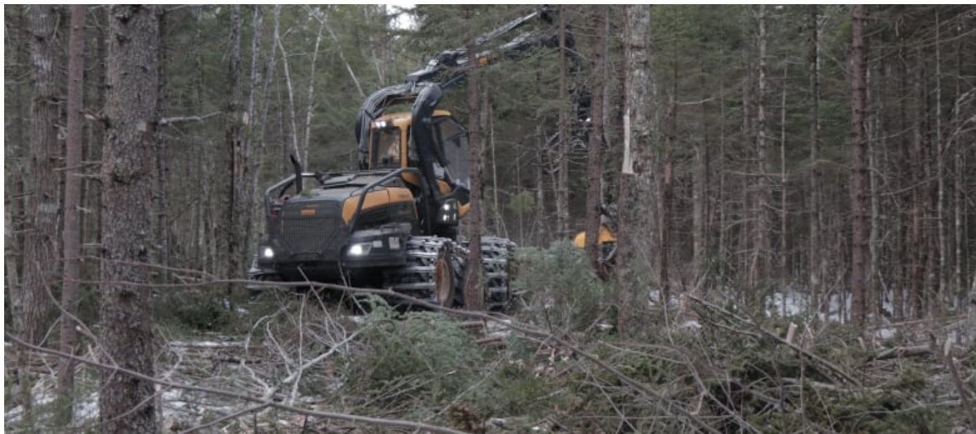
A harvester removes trees during a partial cut in Colchester County. (Michael Gorman/CBC)
