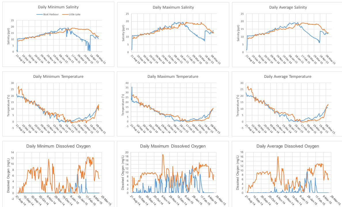
Figure 4.1: Daily Summary of Salinity, Dissolved Oxygen and Temperature from Data Loggers in Little Lake and Boat Harbour in 2014 and 2015
