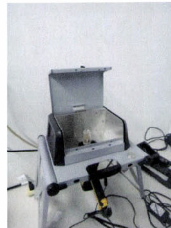
Figure 4-Portable XRF in test stand
