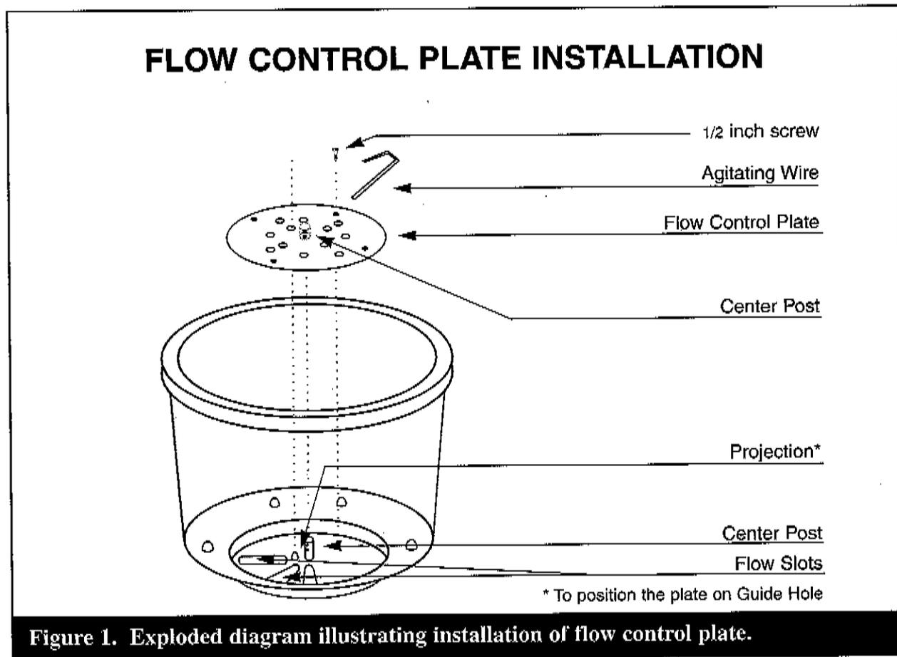
Figure 1. Exploded diagram illustrating installation of flow control plate.
