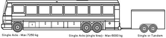
Single Axle (dual tires) - Max 9100 kg Tandem Axle - Max 18,000 kg
