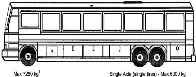
Single Axle (single tires) - Max 6000 kg Single Axle (dual tires) - Max 9100 kg Tandem Axle - Max 18 000 kg
