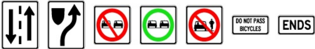
RB-24 60 x 75 cm RB-25 60 x 75 cm RB-31 60 x 60 cm RB-32 60 x 60 cm RB-33 60 x 60 cm RB-33S1 60 x 30 cm RB-33S2 60 x 30 cm
