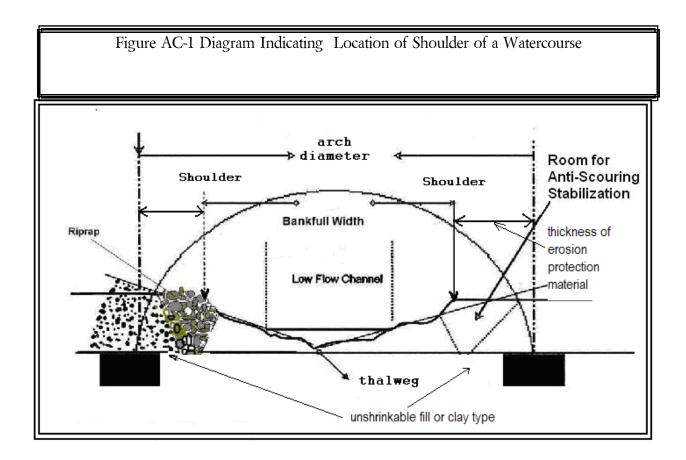
AC10. The natural material located beneath the abutments must be capable of supporting the structure and the loads travelling over it. If the natural substrate material is not capable of supporting the structure, it shall be replaced with granular material capable of supporting the intended loading.
