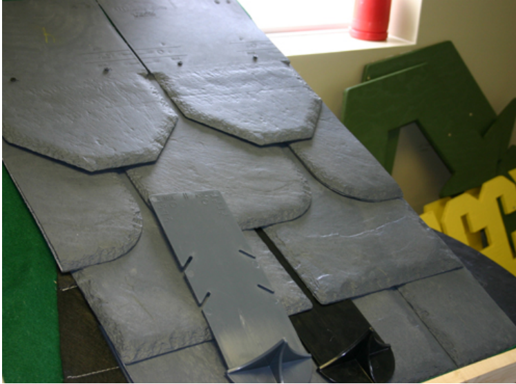
Figure 9. 'Beveled Edge' and 'Beaver Tail' recycled tire and plastic roofing shingle
